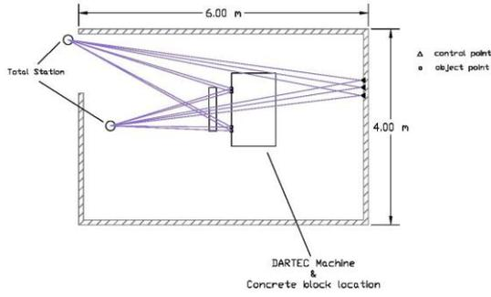
Figure 1. Micro triangulation monitoring network set up in the laboratory (Md Som et al., 2004)
