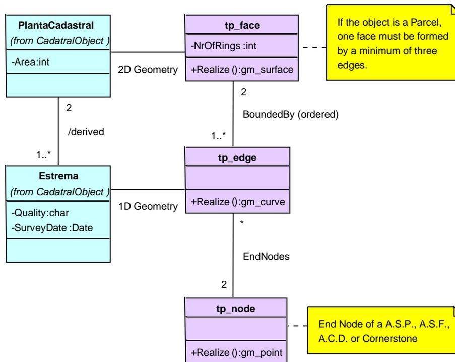
Figure 3: Geometric Cadastre - Geometry and Topology
