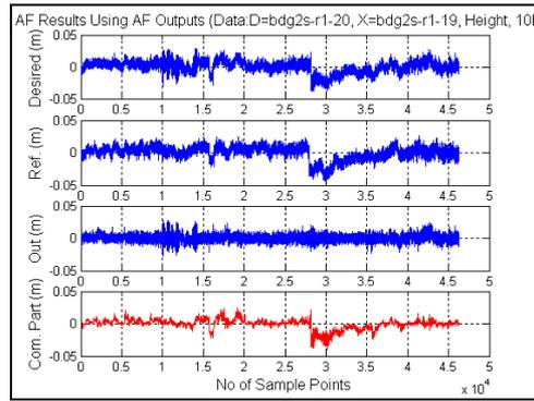
Figure 3 Vertical AF for two days time series for the single frequency rover with dual frequency reference. Desired signal is the coordinates from 20<sup>th</sup> June, reference signal is the coordinates from 19<sup>th</sup> June, the output signal is the bridge movement and the common part is the multipath and cycle slips.
