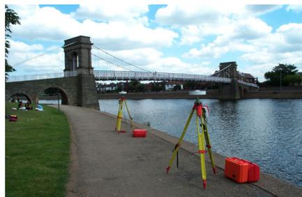
Figure 1 The two riverside reference receivers Ref 1 on the right and Ref2 on the left with the Wilford Suspension Footbridge in the background
