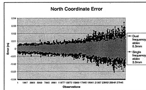
Figure 2 The coordinate error in the north direction for the zero baseline tests
