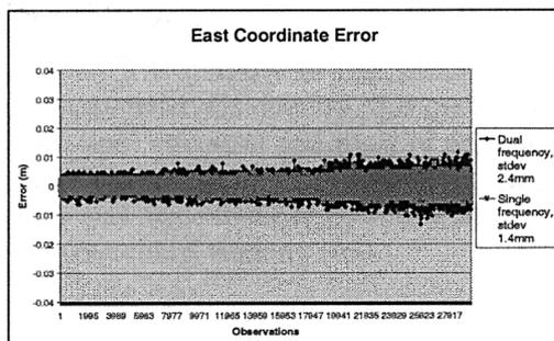
Figure 1 The coordinate error in the east direction for the zero baseline tests
