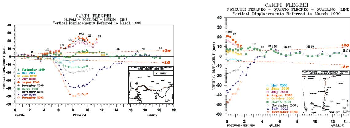
Fig. 10- Vertical displacements at Campi Flegrei, along the E-W line (on the left) and N-S line (on the right) as referred to 1999 survey.
