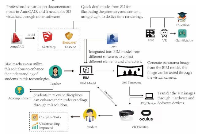
For case study 2 models are created based on AutoCAD 2D drawings (although they could also be created using as-built survey technologies), and then created 3D geometric model in SkechUp. There is a plugin in SkechUp called Enscape that can create a real-time rendering environment for better illustrating the design content. Various interaction between people and the model can be established by multiple visualisation tools.
