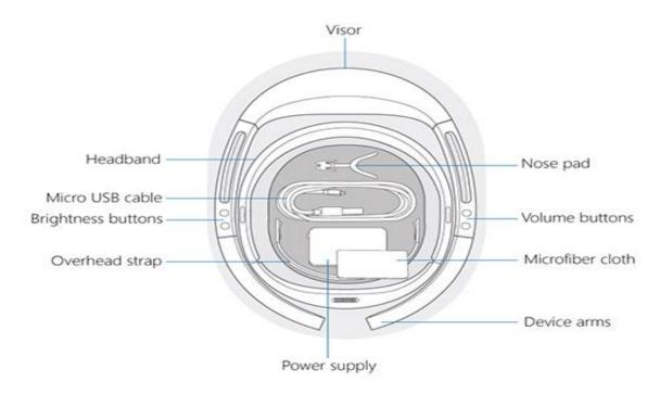
Figure 4 Diagram of the main features of the Microsoft Hololens.
