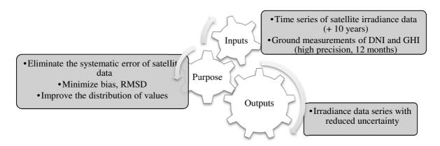
FIGURE 1. Principle of statistical approach of local calibration
