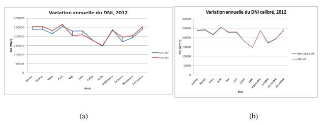
**FIGURE 6.** Comparison between monthly irradiances before (a) and after (b) calibration with in situ measurements for the 2012 common period (case of Ouarzazate station)
