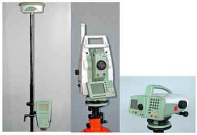
Figure 1: Highly accurate survey instruments: GNSS receiver, total station, level instrument (from left to right), (source: IIGS)
