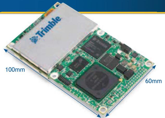
The Trimble BD970 GNSS system is a compact multi-constellation receiver designed to deliver centimeter accuracy to a variety of applications. The Trimble BD970 GNSS receiver supports a wide range of satellite signals, including GPS L2C and L5, GLONASS L1/L2 signals as well as Galileo GIOVE-A and GIOVE-B test satellites for signal evaluation and test purposes.
