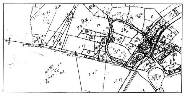
**Figure 5.** Part of an analogue cadastral map from 1983 as used, rectified, and updated over a period of about 100 years. The map is an "island map" and is not linked to a national grid. The display is difficult to interpret, and even though the map was redrawn in 1984, it is not efficient for daily land management. (Courtesy of the National Survey and Cadastre, Denmark).
